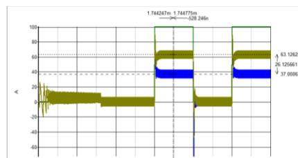
200A load transient over two paralleled stamps with non-symmetric feedback connections
